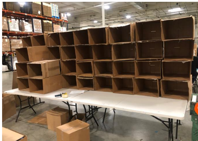
Figure 3: Excessive WIP Cardboard Boxes Wasting Space
